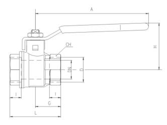
DN shows the nominal flow diameter. Actual flow diameter complies with full port DIN 3357 part 4. Stem configuration of valves over 2" is slightly different. Ask for details at our Service Center
